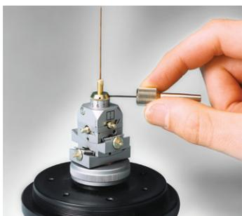
Figure 27. Capillary sample mounted on goniometer head
