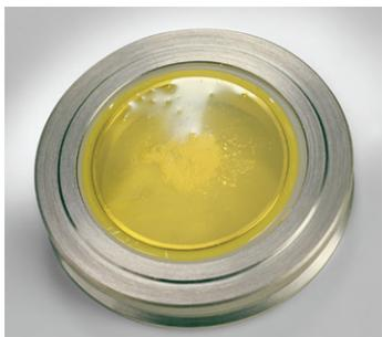
Figure 26. Sample holder for transmission measurements
