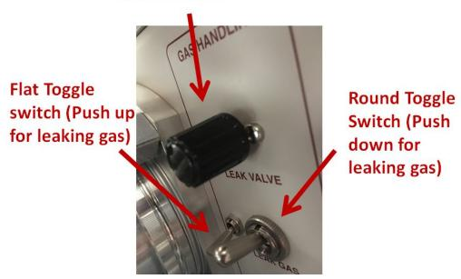
Behind the Carbon Coater unit (left side while facing machine) is the gas handling controls. The flat switch is down and the round switch is up when not leaking gas (closed).
