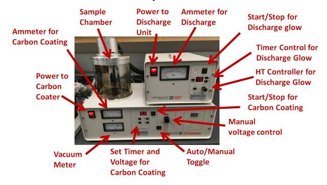
Front Panel - Top unit (Power Unit) is for discharging specific metal Front Panel - Bottom unit (Carbon Coater) is for evaporating carbon.
