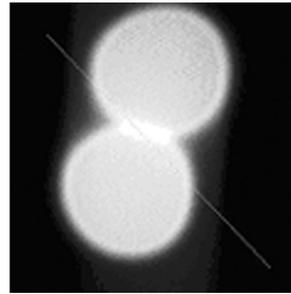
Misaligned beam tilt pivot
