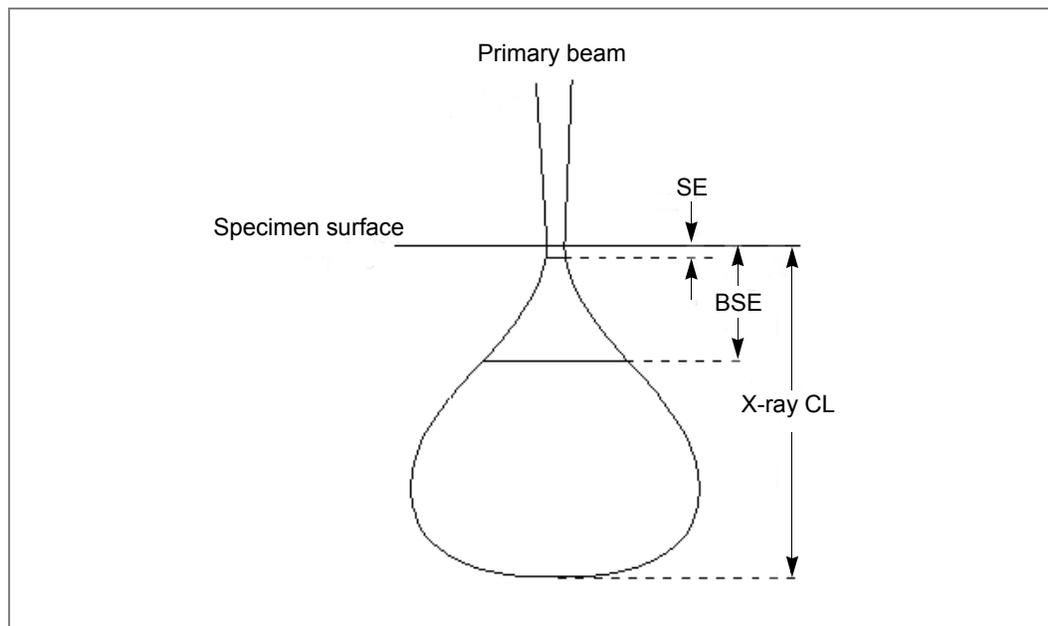
However, for electron transparent specimen, the thickness is so small that the beam is only slightly broadened before it comes out of the sample. The same argument holds for the applications using the transmitted electrons, such as EELS, CBED and STEM. Because of this, beam broadening, a serious problem for spatial resolution in SEM is not very crucial in TEM as long as the specimen is thin.
