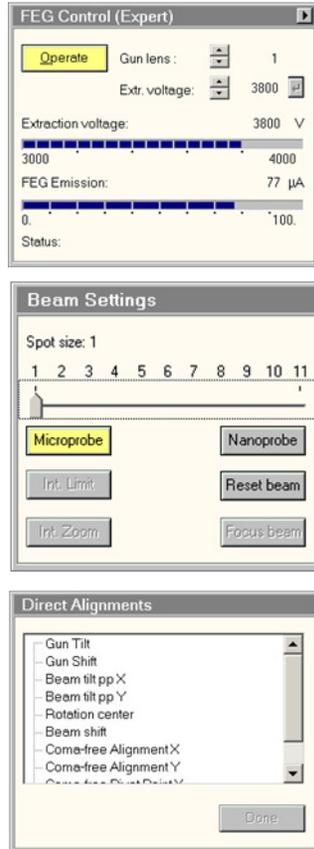
2. Select gun lens 2-5, spot size 3 and Microprobe, or recall a FEG register. If gun lens was changed, do gun tilt and gun shift on direct alignments.
