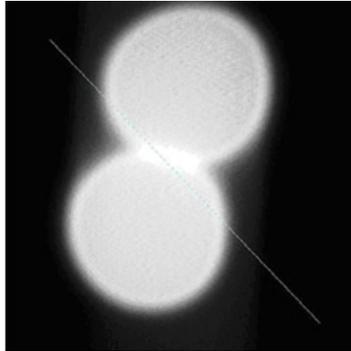
Misaligned beam tilt pivot points
