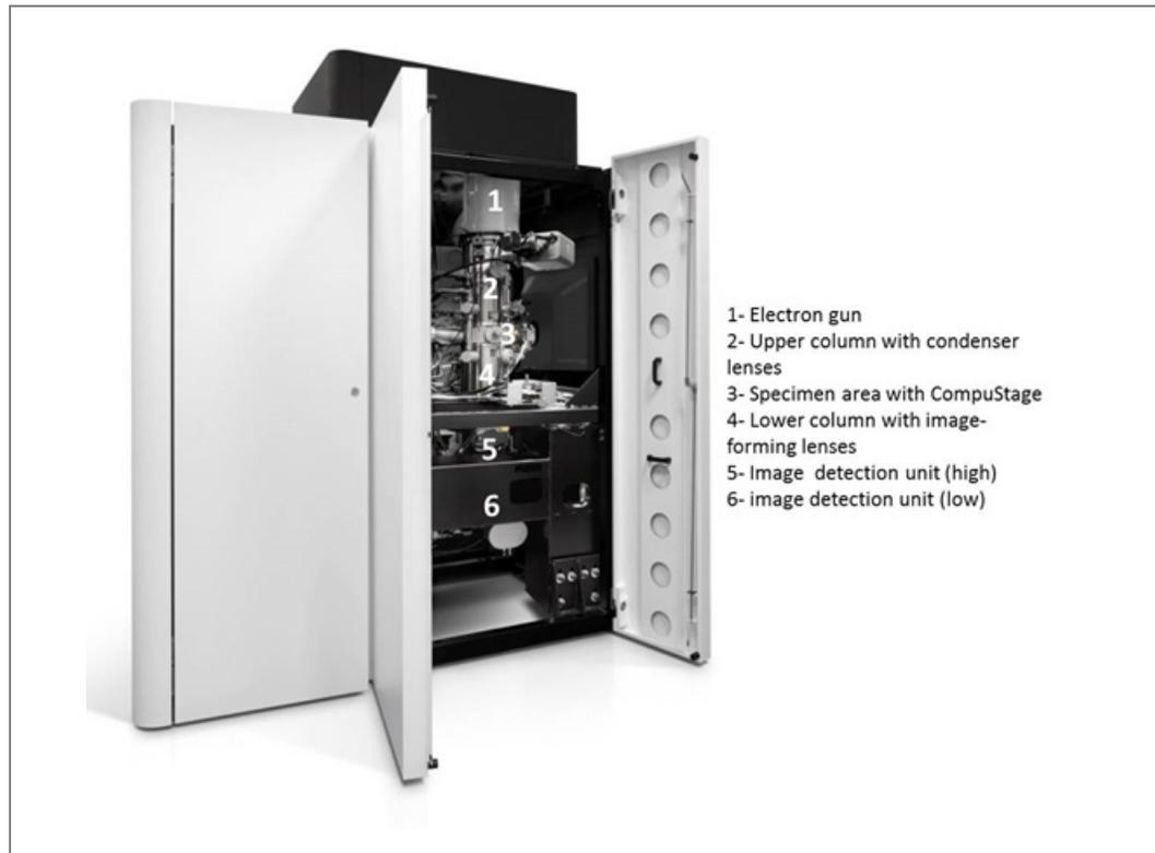
Basically, the microscope consists of the following elements, which are also noted in *Figure 34*:
