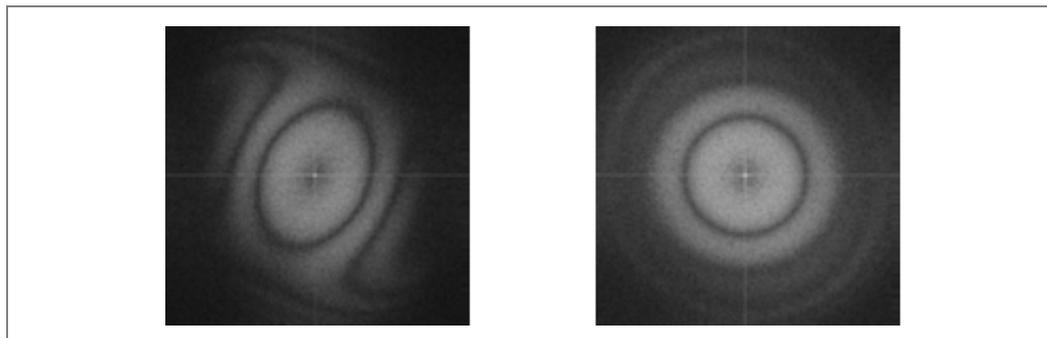
Stigmators are aligned by small procedures as mentioned above. If they are misaligned, the astigmatism correcting operation will create a shift in image/spot. To correct astigmatism, you need a well aligned stigmator; to align a stigmator, you also need small astigmatism. Therefore, you should occasionally perform the following sequence: correct astigmatism, align stigmator, and correct astigmatism again.
