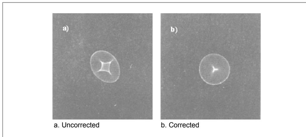
The objective lens astigmatism is an important factor for image quality. For high resolution work, it may even cover the feature of atomic structure. To minimize objective lens astigmatism acquire a live image of an amorphous area on digital camera at enough high magnification ( $> 100 \text{ kx}$ ) with live (reduced) FFT. Stigmatize to get round features at approximately 100 nm defocus; 1-2 rings visible (see [Figure 70](#)).
