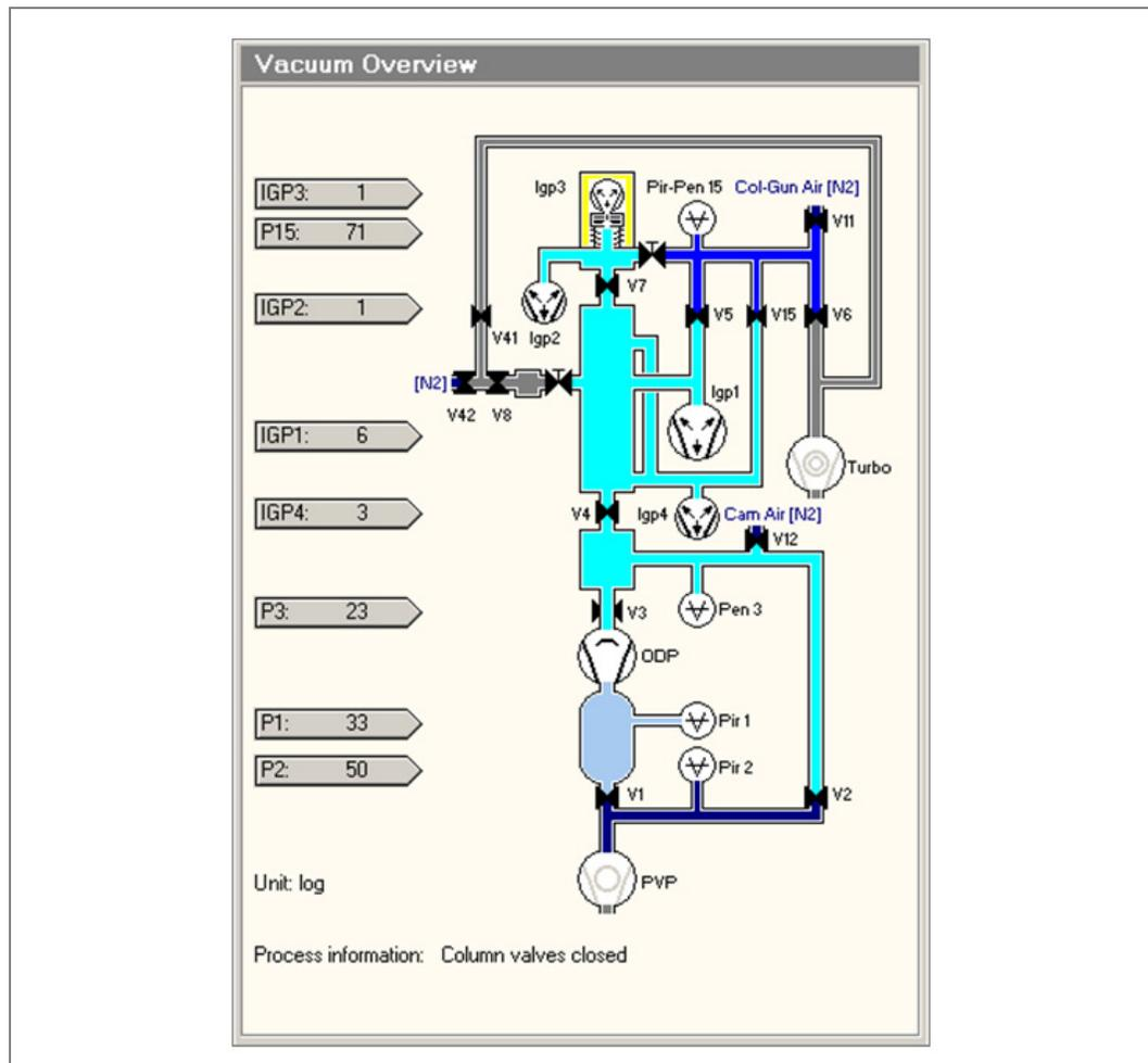
One extra pump (IGP4) evacuates the liner tubes that connect the projection chamber to the specimen area and the specimen area to the gun. Further, the electron gun (FEG) is pumped by IGP2 (gun area) and a small IGP3 (emitter area). FEG microscopes are also equipped with a TMP to pre-pump the column and to pump on the specimen air-lock.
