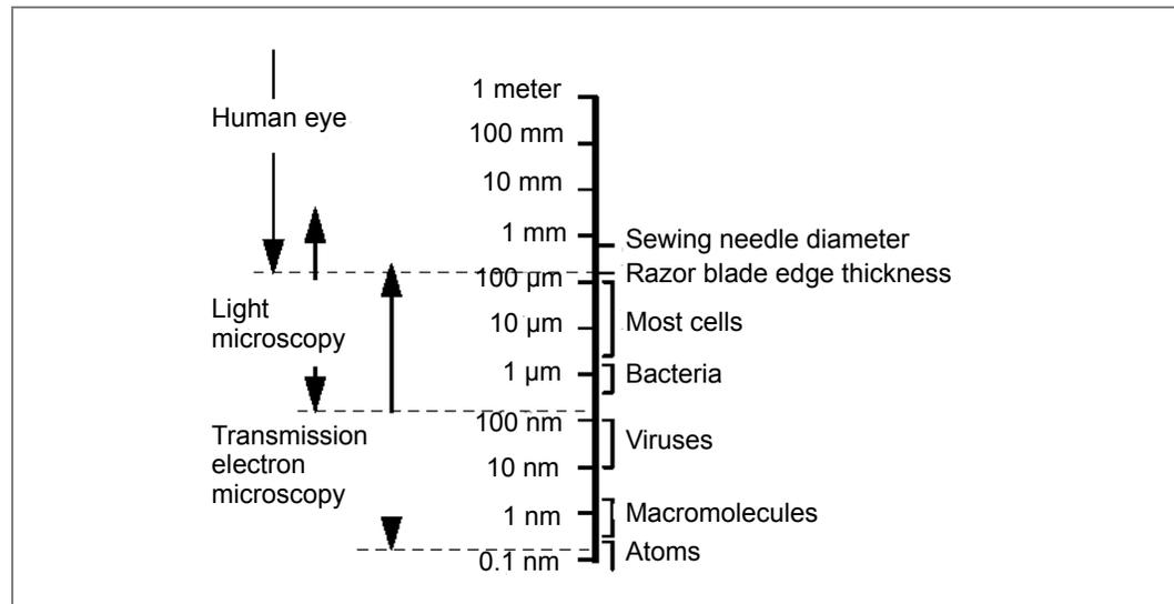
In principle, the resolution of electron microscopy can be improved by increasing the high tension, as the following relation between the wavelength ( $\lambda$ ) and the high tension (U in volts) holds.
