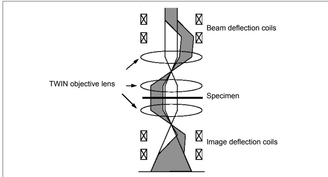
For example, in the Focus state (see shaded ray-path) an off-axis area in a specimen is illuminated by the beam deflection coils and its image is shifted to the center of the viewing screen by the image deflection coils. In the Exposure state, neither the beam nor image deflection coils are activated, so the area around the optic axis is imaged.
