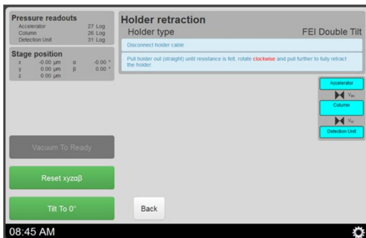
2. When 'Auto reset stage' has been enabled in the settings screen, the stage is reset to 0,0,0,0,0 automatically. Additionally, buttons are available to reset the stage, or to rotate the stage to -55 degrees (this button toggles between -55 and 0 in order to aid with retracting a cryo holder).
