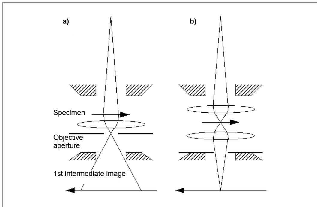
Imaging proceeds as follows: At the back focal plane of the lens, a diffraction pattern is formed; further down the column, the first intermediate image is at the image plane. This image plane is also called the selected area plane, where the selected area (or diffraction) aperture may be present. The objective aperture is positioned in/near the back focal plane of the objective lens.
