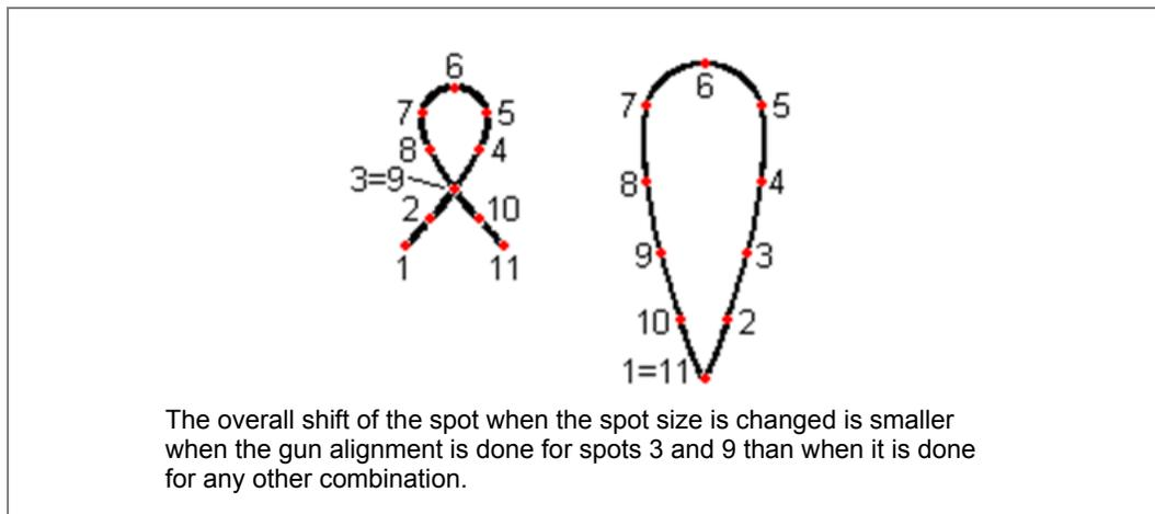
In this way, the electron beam is aligned along the optical axis, and a spot displacement when changing spot sizes is minimized. In an additional step, this displacement can be further minimized by aligning all other spot sizes as well (spot size-dependent gun shift).
