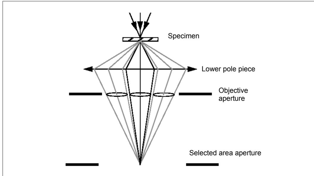
In Microprobe mode, a micro-diffraction pattern is obtained using a condensing beam. The pattern consists of broad disc-like spots rather than sharp points due to the large convergence of the incident beam. The disc shape of a diffraction spot actually represents a range of the simultaneous illumination angles (*Figure 53*).
