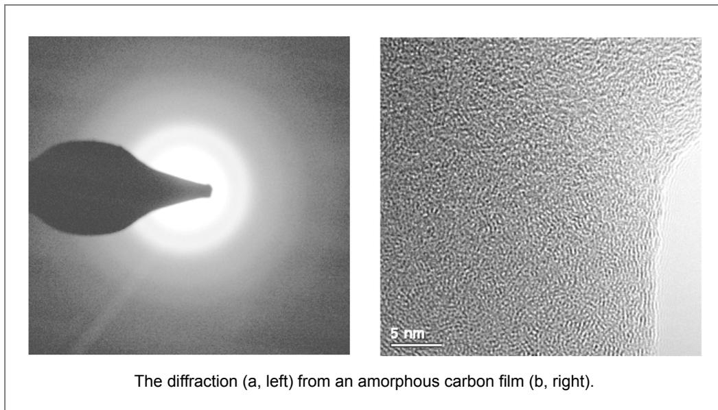
Figure 64 shows the diffraction pattern (a) from an amorphous carbon film (b). A diffuse ring can be observed, which reflects its amorphous nature. In fact, it relates to the nearest C-C atomic distance of 0.34 nm. Due to the amorphous nature, no clear crystalline fringes, like those in Figure 62b, may be observed in Figure 64b.
