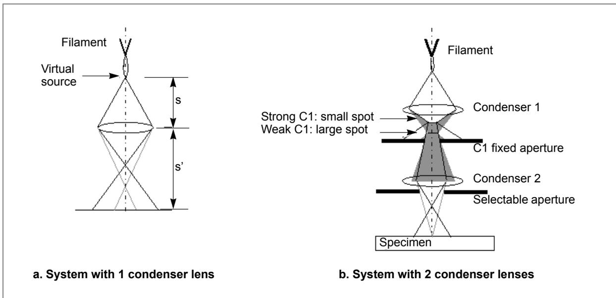
For many applications, microscopists use various spot sizes. This is achieved by working with another condenser lens (*Figure 38b*).
