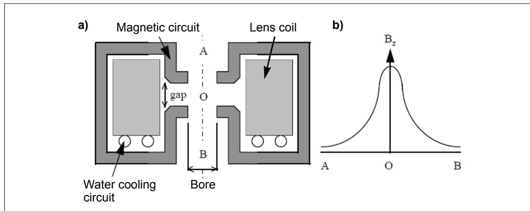
With a given lens geometry, the strength of the field in the pole piece gap is proportional to the excitation of the lens, defined as the product of current  $I$  in the windings and number of turns  $N$  in the coil:
