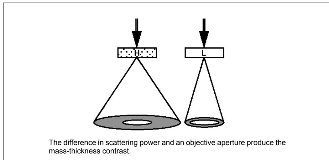
*Figure 56* is a schematic representation of this contrast mechanism, where the specimen region with higher scattering power is labelled H and the lower one marked L. More electrons are scattered to higher angles by H than by L, though the electron distribution declines quickly with the angles. The total number of electrons reaching the base plane of the illumination cone in *Figure 56* is the same for both regions, as long as both are equally illuminated by the incident beam.
