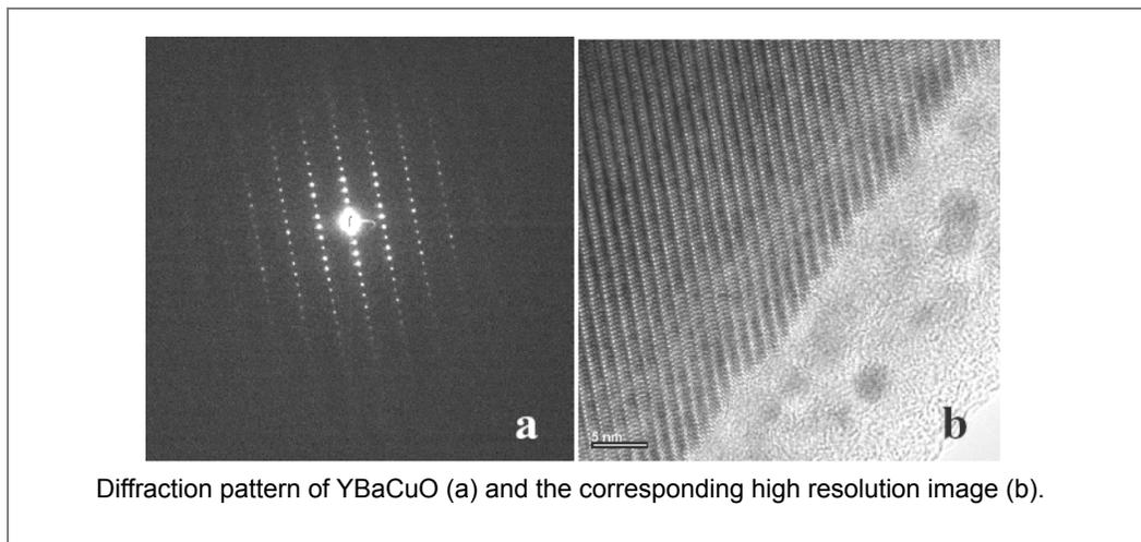
In *Figure 62*, “a” is a typical diffraction pattern obtained from superconductor YBaCuO recorded with a CCD camera, and “b” is a corresponding phase contrast TEM image showing the crystalline fringes. In the diffraction pattern, the central spot (the forward direction or  $2\theta = 0$ ) is so strong compared to the other spots that the CCD pixels were actually saturated and artifacts may be observed. The largest Bragg angle with recognizable intensity in *Figure 62a* is  $< 2^\circ$ .
