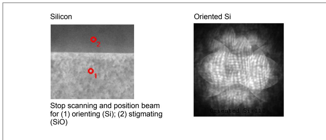
14. Orient the region of interest (position 1 in *Figure 81*) to be accurately on zone axis according to its diffraction pattern. Silicon pattern in  $\langle 110 \rangle$  with slightly underfocus is shown.
