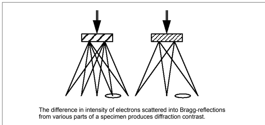
Diffraction contrast is widely used to study defects in crystals, because the regions around the defects have Bragg angles differing from the perfect crystalline matrices and thus produce contrast to be observed.
