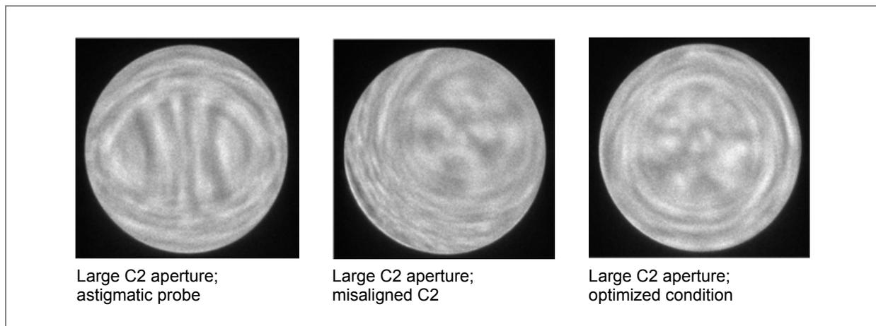
18. Change the condenser C2 aperture to a larger one, e.g., 150  $\mu\text{m}$ . A larger Ronchigram is now visible, which makes it easier to tune. Focus, stigmatate, and align the aperture based on the Ronchigram.
