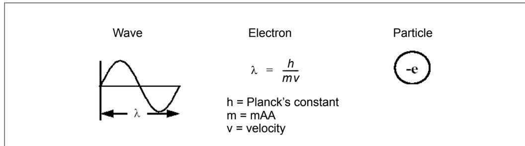
In both light and electron microscopy the ultimate obtainable resolution is limited by the wavelength. In a light microscope, small points with dimensions similar to the wavelength of light are imaged as ring patterns with an intensity distribution such as that shown in *Figure 5*.
