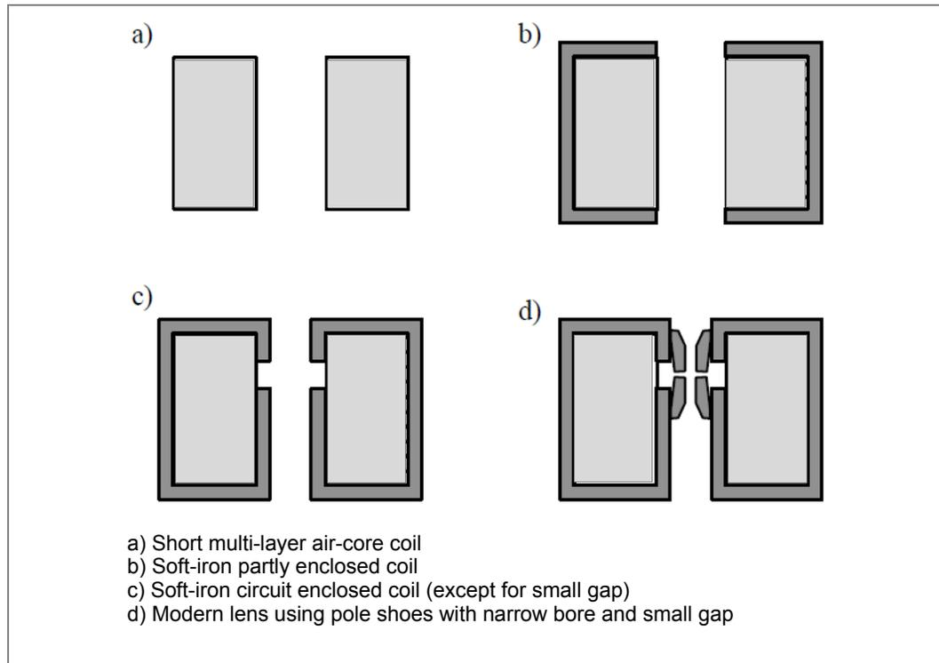
One of the most important features of an electromagnetic lens is the fact that its focal length can be changed simply by changing the lens current. This enables you to adjust the lens system, i.e., focusing and magnification, without any mechanical change.
