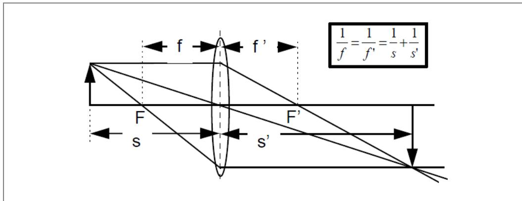
Figure 10 shows the typical ray paths and image formation analogous to a glass lens.
