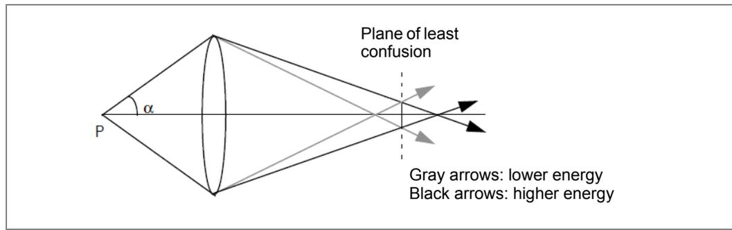
The chromatic aberration results when waves of different energies converge at different focal planes. In an electromagnetic lens, electrons with shorter wavelength, and thus more energetic, have a longer focal point than do electrons with a longer wavelength.
