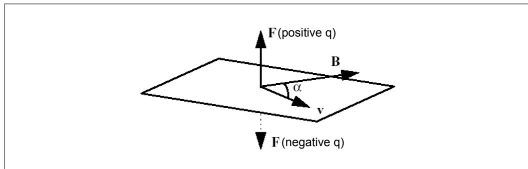
When the electron moves in a region where there is an additional electrical field  $\mathbf{E}$ , the total force is the sum of the electric force and the magnetic force:
