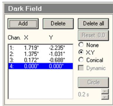
There are two ways for beam tilting: X-Y and Conical (Dynamic Conical Dark-Field is available to Talos systems with STEM functionality). The beam tilts are set with the **Multifunction-X**, and **Multifunction-Y** knobs on the left and right-hand control pads.
