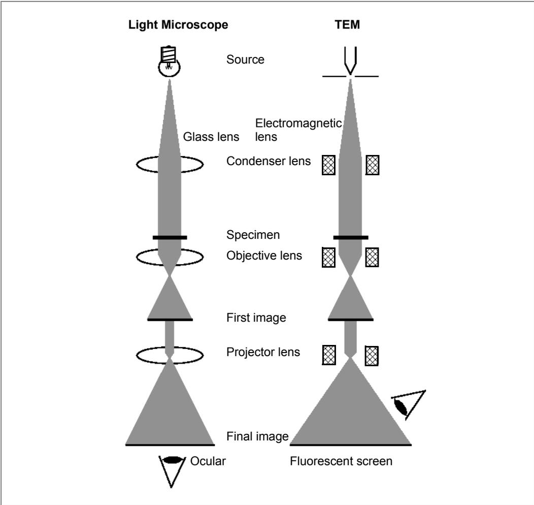
*Figure 1* compares a light microscope and a transmission electron microscope. The principle is essentially the same: a source illuminates the thin specimen with the aid of a condenser lens, and then the objective lens produces an image that is subsequently further magnified by the projector lens. The three major differences are:
