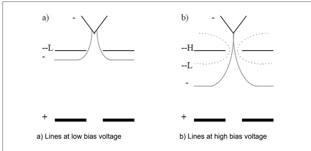
The emitted electrons that pass through the Wehnelt aperture are focused into a crossover between the Wehnelt and anode. This crossover acts as the electron source for the optics of the microscope. The size of the crossover is determined by the type of filament as well as by the bias.
