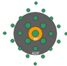
Alignment of diffraction pattern on BF/DF
