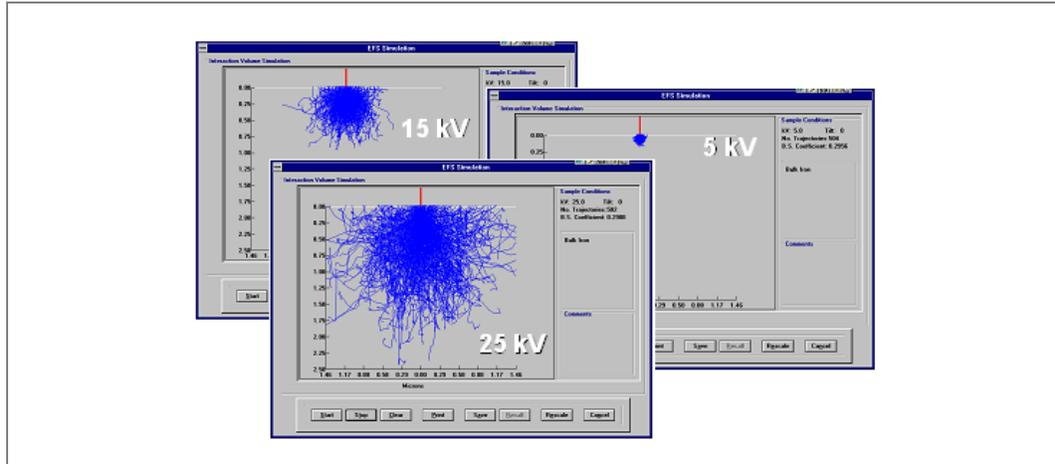
It is from Monte-Carlo simulations, which take account of both elastic and inelastic multiple scattering and model the trajectory of a single electron based on the probability of scattering angles and energy transfer.
