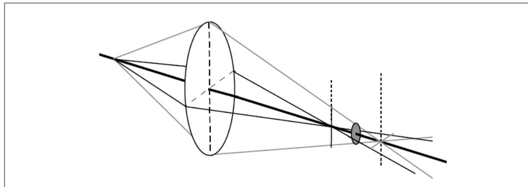
Astigmatism is caused by the imperfections in the objective lens: imperfection of the circularity in the bores, flatness of the pole faces, and asymmetry in the magnetic material are the main reasons. However, the specimen itself and contamination can also change the symmetry of the magnetic field and induce astigmatism. Fortunately, astigmatism can be corrected with stigmators, which compensate the asymmetry and will be described in detail later.
