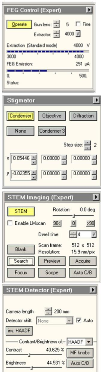
2. If necessary, store the current TEM gun alignment in the FEG register for convenience.
