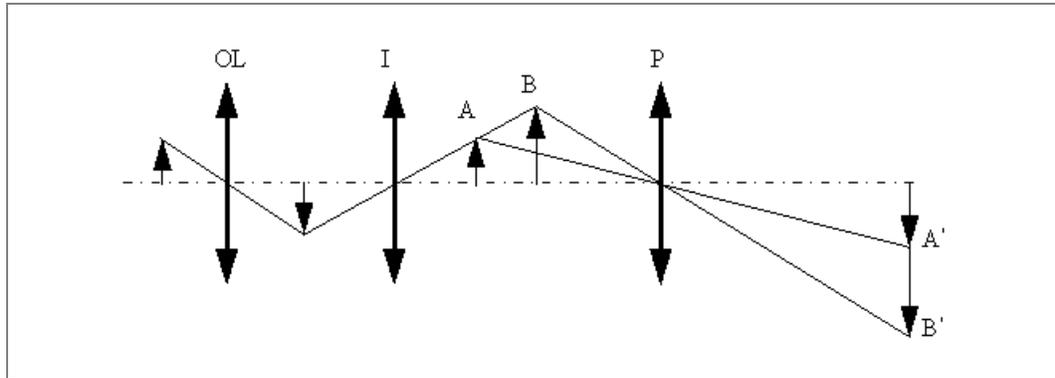
The additional information (diffraction pattern) at the back focal plane of the objective lens can be imaged by turning down the current through the intermediate lens, enlarging its focal length, and focussing the imaging system to that plane. When the imaging system focuses on the selected area plane, the M/SA mode, on the viewing screen we see the enlarged image; when it focuses on the back focal plane, the D mode, we see a diffraction pattern.
