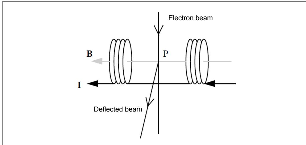
In principle, a more or less uniform magnetic field  $B$ , perpendicular to the incident electron beam and generated by the current through the coils, acts on the electrons and deflects them. The combination of two such coil pairs perpendicular to each other can deflect a beam in any direction. The point where the direction of the beam is changed is called a *pivot point*, and the beam “pivots” or “tilts” at the point.
