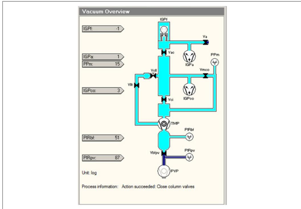
At the bottom, it starts with the rotary pump (PVP). Above the PVP is the buffer tank that is separated from the PVP by a valve (Vbfpv). Pir (Pirpv and Pirbf) are Pirani vacuum-pressure measuring gauges. Valve Vci separates the projection chamber from the upper part of the column.
