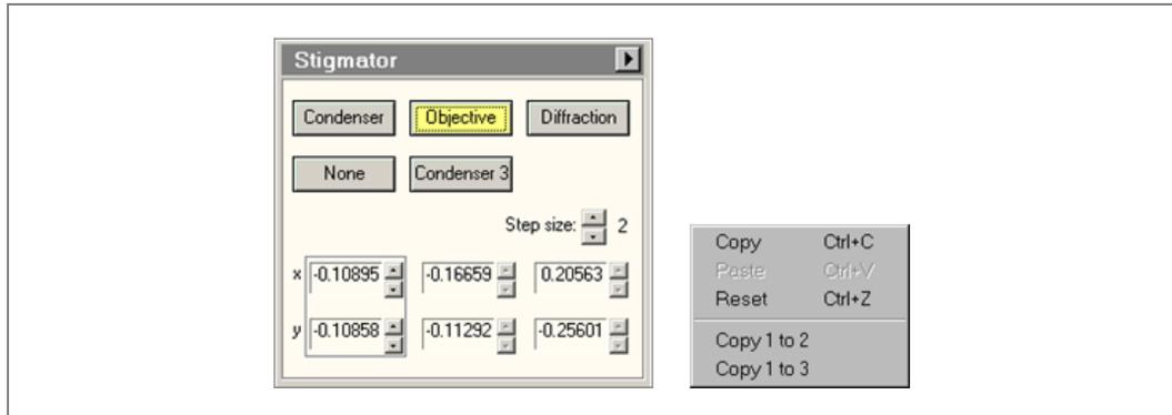
Stigmator settings can be stored in three channels, copied, and reset (zero settings). The active channel is outlined by a frame. The criteria for astigmatism correction are summarized in *Table 10* (see also Talos online help *Astigmatism Correction*).
