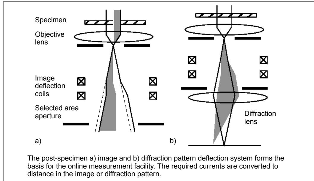
The measurement function is carried out by determining the image/diffraction pattern shift (given by the currents in the deflection coils) that is needed to adjust the points of interest onto a reference point. You must perform a calibration using a specimen with known dimensions in advance.
