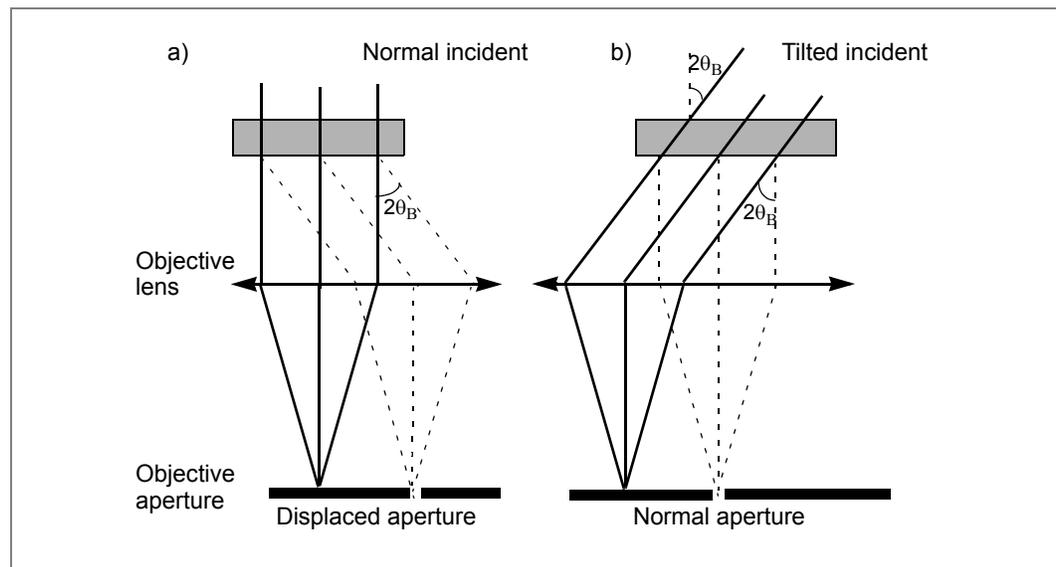
[Figure 51](#) shows dark-field imaging by (a) displacing the objective aperture and (b) tilting the incident beam. Only one diffracted beam is shown in the figure.
