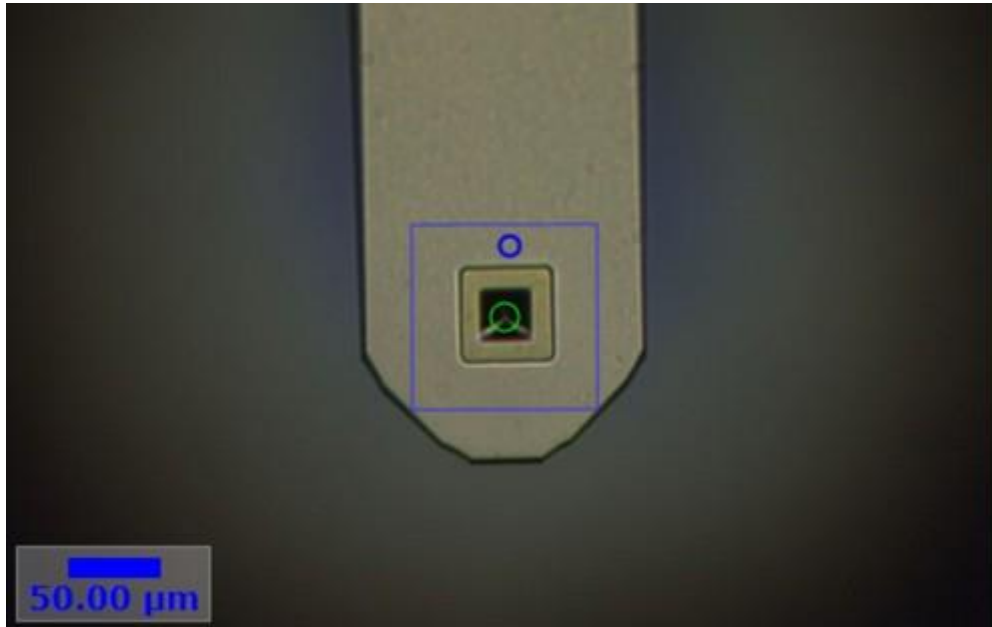
Fig. 1: SNOM cantilever focused into the aperture (top view)
