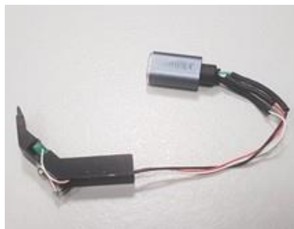
Figure 1: Cantilever connected with silver conductive paint (left) and EFM arm with electric connection (right)
