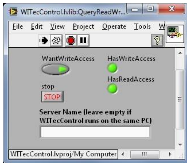
Fig. 2: Testing the Read and Write access of LabVIEW for WITec Control.
