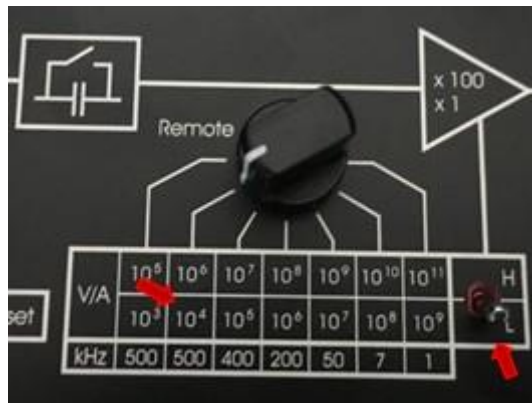
Fig. 1: Example of the amplification setting of the femto current amplifier.
