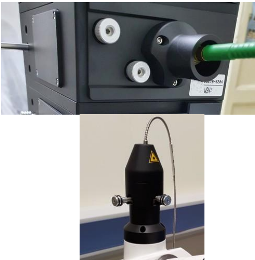
Figure 2: Fiber alignment screws (left: starting 2015, right: before 2015)
