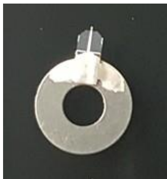
Figure 1: Cantilever connected with silver conductive paint (left) and EFM arm with electric connection (right)
