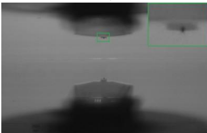
Fig. 1: SNOM cantilever in rear view with reflection on the sample surface.
